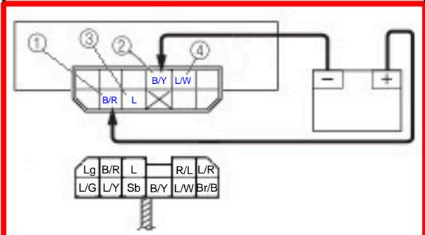
Does the starting circuit cut-off relay have continuity between blue and blue/white?
